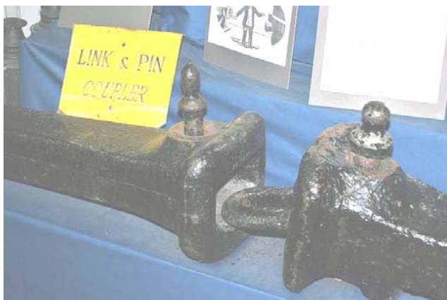
Fig. 737 – Enganche link-and-pin
