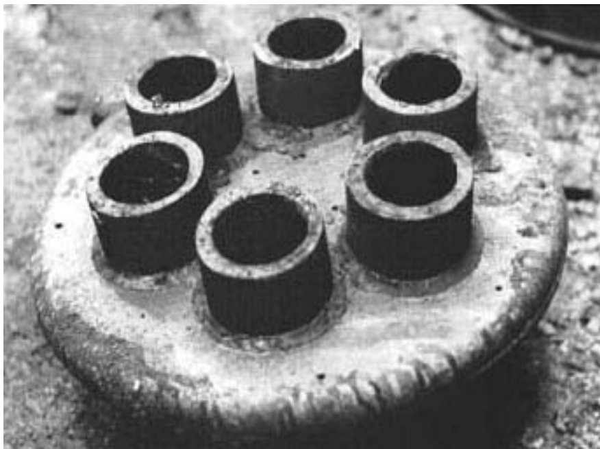
Fig. 218 – Tobera de escape Peeperpot
